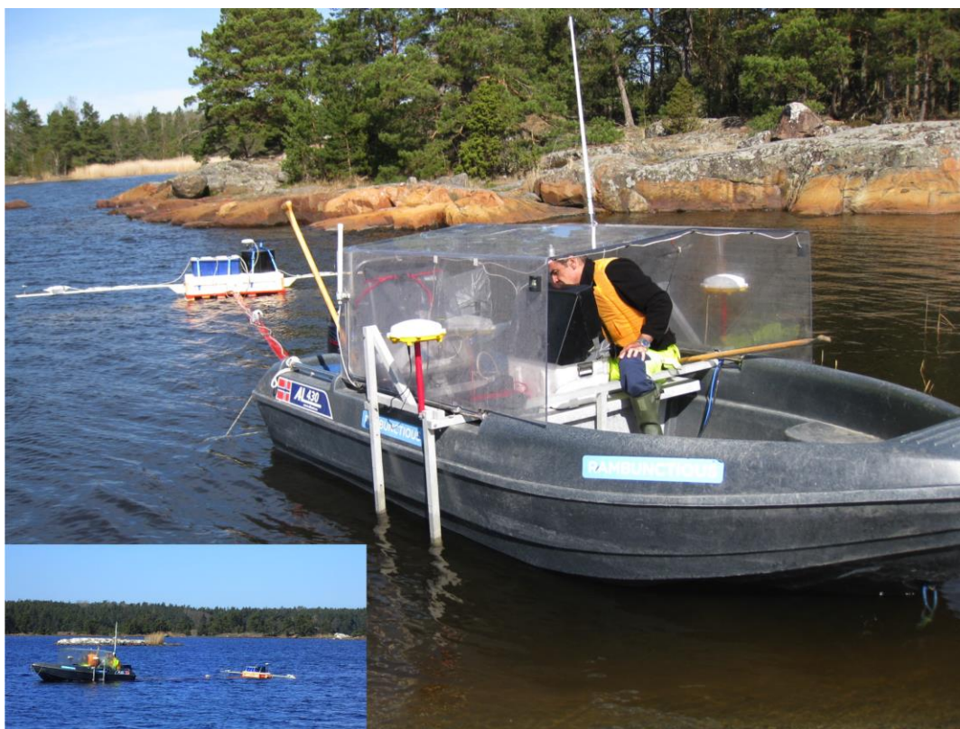
Figure 13. Photos showing the deployment of the boat-towed RMT system during the Äspö experiment.
